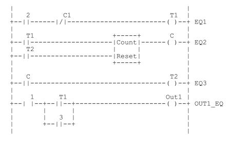
Rung T1 is equation 1. The pulse time must be set to the allowable on time for the locked rotor condition to prevent tripping the overloads, in this case 2.5 seconds.
